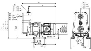
\*) Dimensions for SBM315, SBM315/60Hz \*\*) Dimensions for SBM315/60Hz
