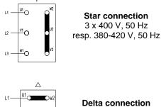
Delta connection 3 x 230 V, 50 Hz resp. 220-240 V, 50 Hz
