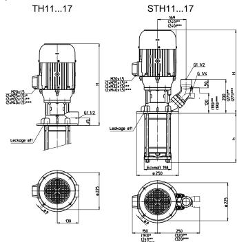
\*) Dimensions. for 7.5 to 10.3 kW ; \*\*) Dimensions for 11.0 / 13.0 kW and 15 kW 60 Hz
