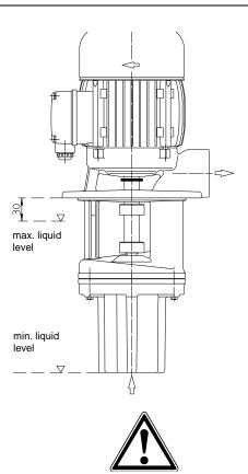
If the pump should lock up and cease, shut pump down (see 6.2) and disconnect from power supply. Pump must be uninstalled and removed from the system prior to its repair.
