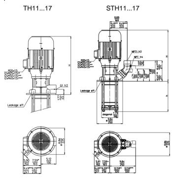
Dimensions in Inches / mm  $^*$ ) Dim. for 11.5. HP to 13.8 HP ,  $^{**}$ ) Dim. For 16.9 HP to 20.1 HP  $^{***}$ ) Dim. Up 25 HP
